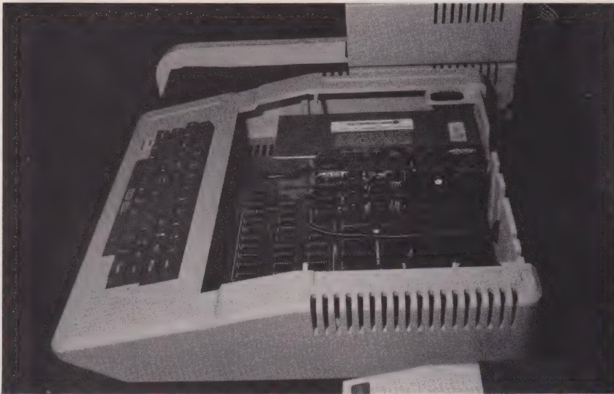
The SoftCard is the PCB closest to the camera in this shot. The disc controller card will be re-fitted in front of it.
